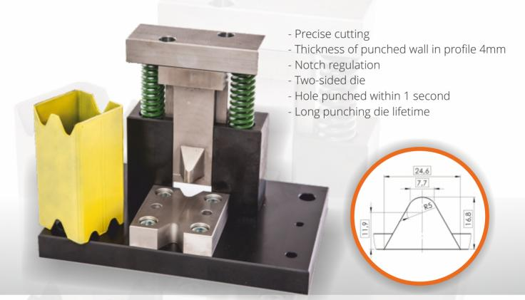
The use of technological notches eliminates air cushions in designs. Thanks to this, the detail is perfectly galvanized, and excess zinc on edges is reduced.
